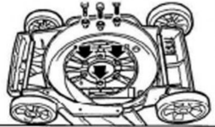
MOTOR MOUNT: (Bottom View) Items 50, 51 assembled in 3 locations indicated.
