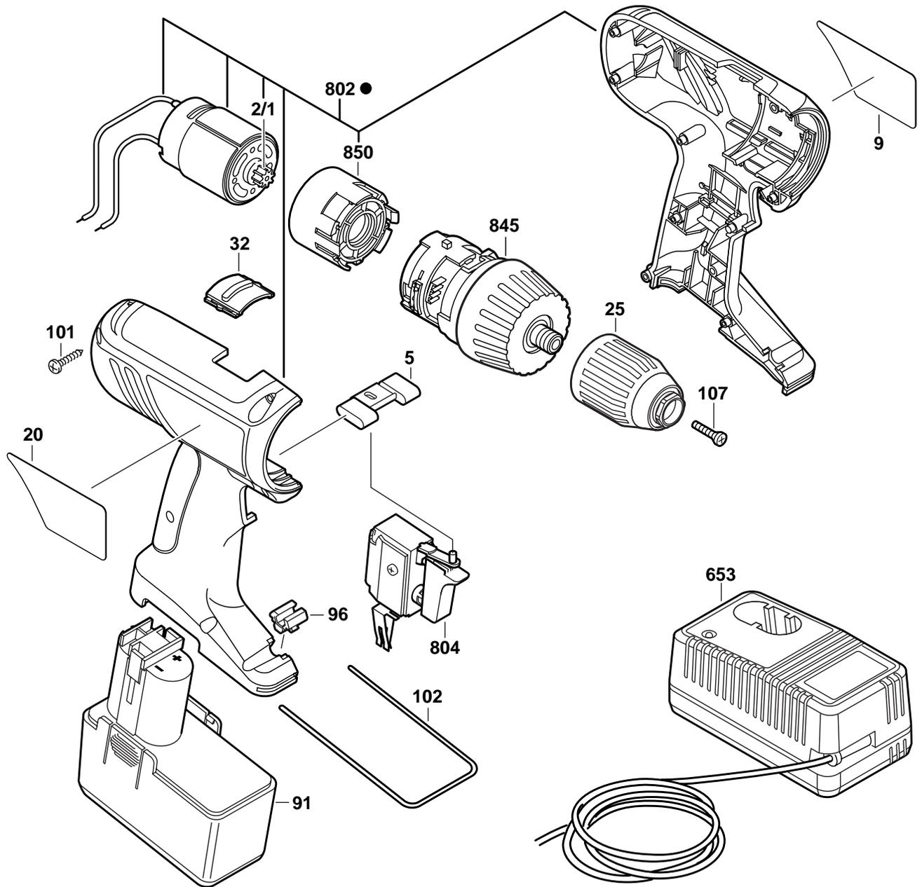
● Pos. 802, Part Number 2 607 022 983, Motor Assembly, now includes the components (Motor Housing, etc.) as pictured above. Older inventory included only the Motor and Pinion Gear, and can be used unless the Motor does not properly fit into the Motor Housing of the subject tool.
