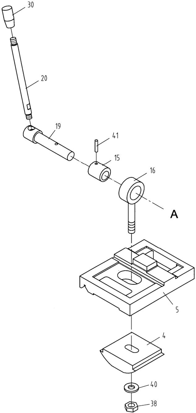
19.2 Tailstock Assembly II – Parts List
