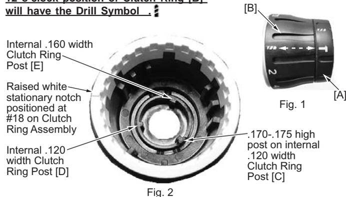
Picture shown with hammer symbol **T** aligned with drill symbol **.** ready for assembly.
