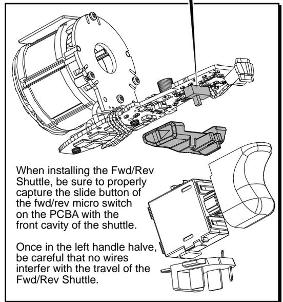
When installing the Fwd/Rev Shuttle, be sure to properly capture the slide button of the fwd/rev micro switch on the PCBA with the front cavity of the shuttle.
