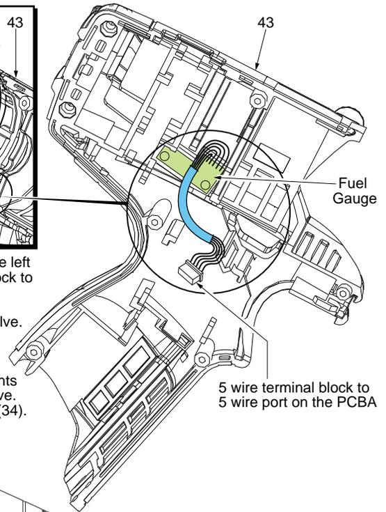
5 wire terminal block to 5 wire port on the PCBA
