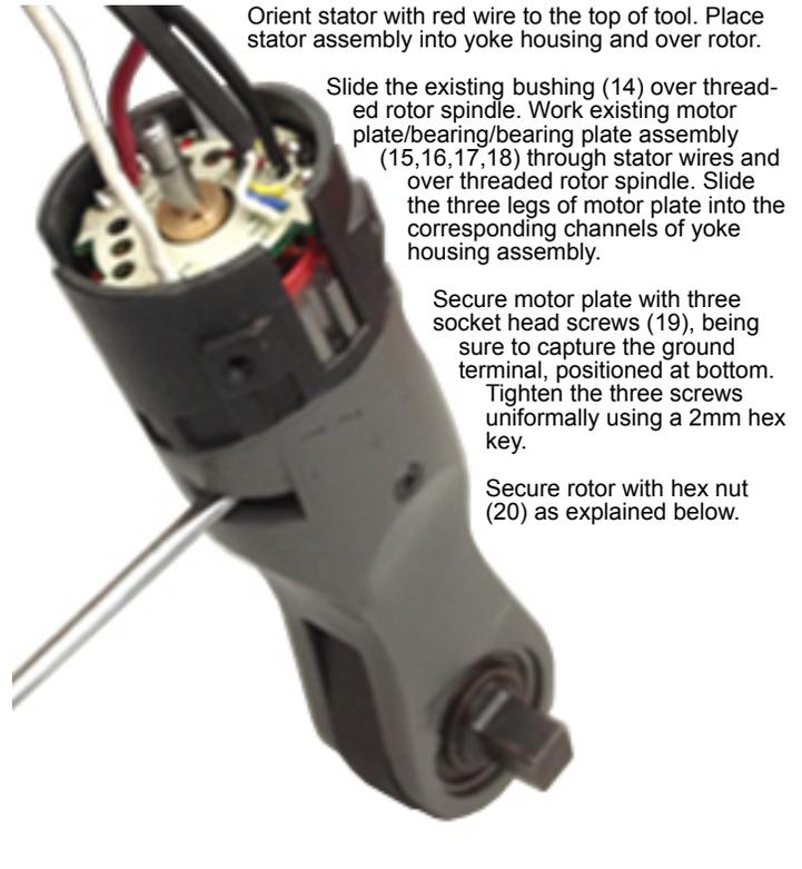
Orient stator with red wire to the top of tool. Place stator assembly into yoke housing and over rotor.
