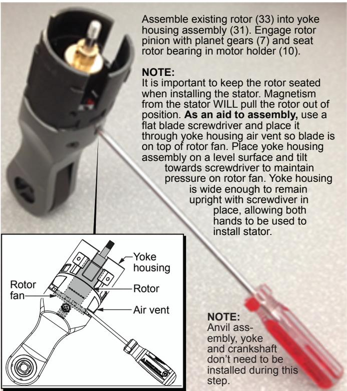
Assemble existing rotor (33) into yoke housing assembly (31). Engage rotor pinion with planet gears (7) and seat rotor bearing in motor holder (10).
