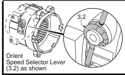
Orient Speed Selector Lever (3.2) as shown
