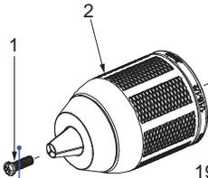
Apply Blue Loctite® thread locking sealant or the equivalent to the threads of the chuck screw (1) before securing chuck to the gearcase spindle. Torque to 90-100in/lbs (7-8ft/lbs).
