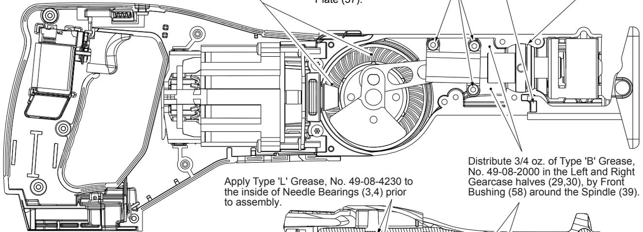
Apply Type 'L' Grease, No. 49-08-4230 to the inside of Needle Bearings (3,4) prior to assembly.
