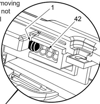
Before installing or removing Armature, to prevent damage to the brush tubes or commutator, push / move Brush Tubes (25) flush to inside brush tube openings of Motor Cage (35) prior to removing the Armature from Motor Cage (35) / Field (22).
