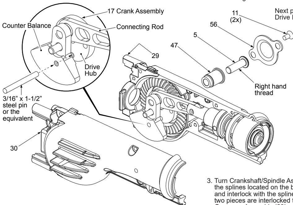
Next place a 3/16 hex key into Drive Hub Bolt (5) and turn Drive Hub Bolt slowly in a counter-clockwise direction until 3/16" steel pin rest against Connecting Rod. 3/16" hex key can now be turned counter-clockwise to loosen and remove RH Drive Hub Bolt (5).
