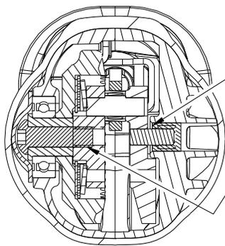
Press Needle Bearing (4) .030" minimum subflush.
