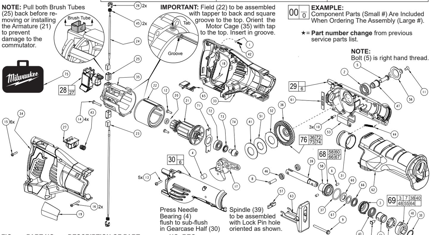
Press Needle Bearing (4) flush to sub-flush in Gearcase Half (30)
