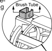
**IMPORTANT:** Field (22) to be assembled with taper to back and square groove to the top. Orient the Motor Cage (35) with tap to the top. Insert in groove.
