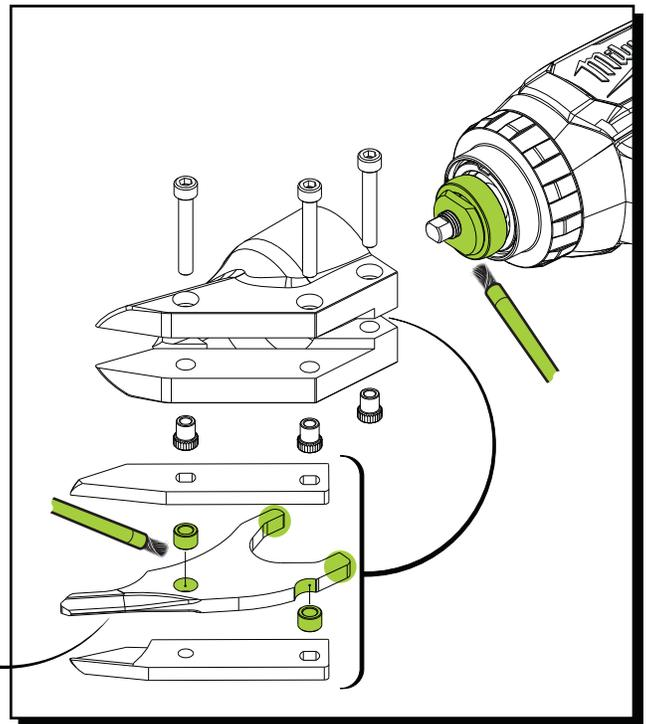
**REMOVING SHEAR HEAD ASSEMBLY FROM TOOL**
