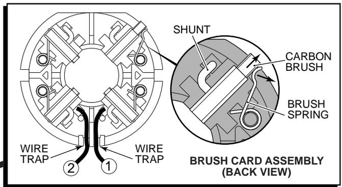
Be sure to place black wire #1 and red wire #2 firmly in the wire traps on the bottom of brush card to prevent pinching between handle halves and end cap.
