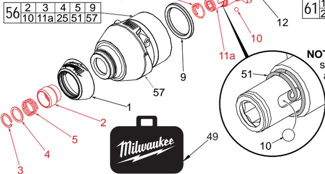
**NOTE:** Place anvil spring (51) onto anvil (11a) with curled end inserted in slot of anvil as shown. Place ball (10) in anvil slot in front of spring.
