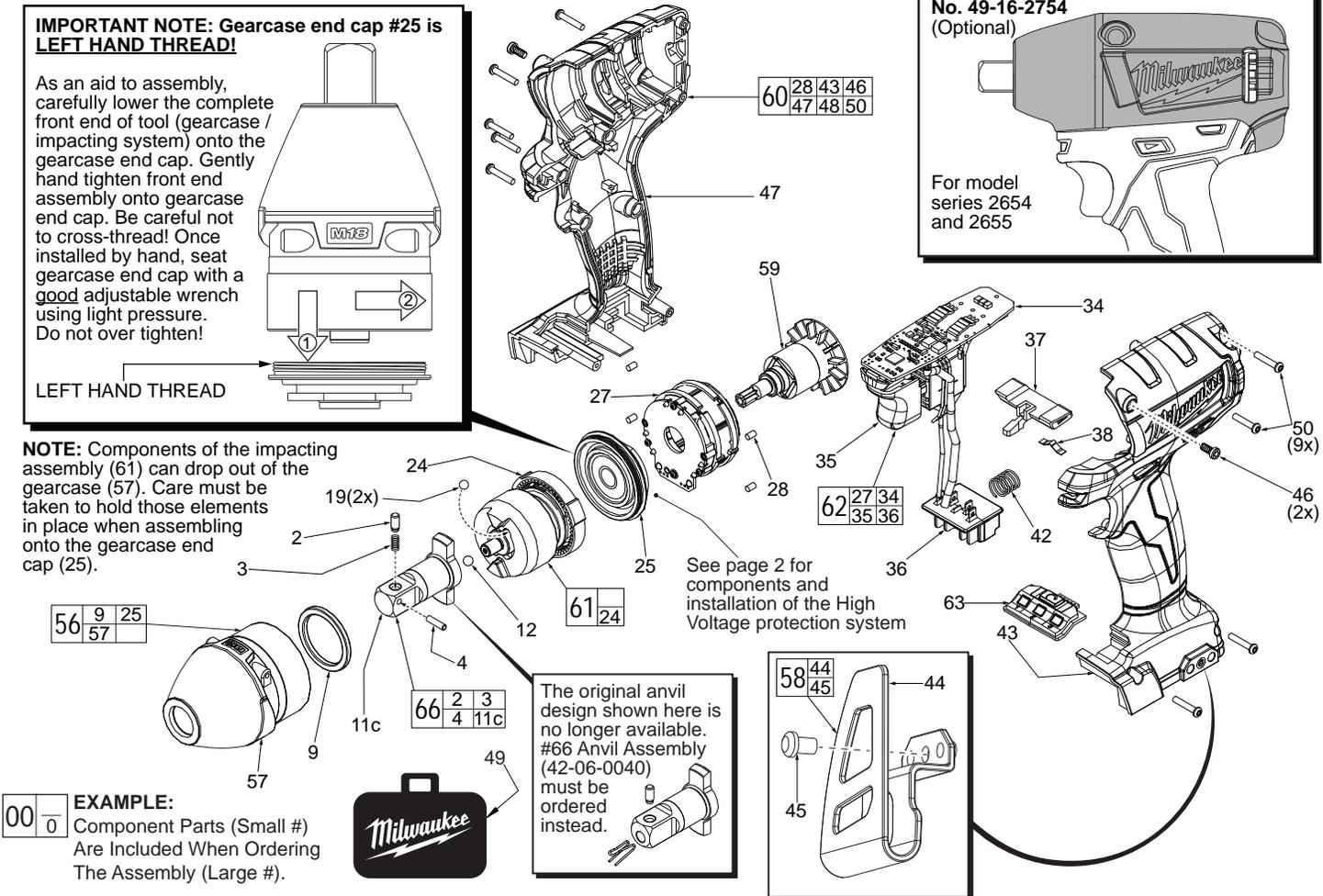
See page 2 for components and installation of the High Voltage protection system
