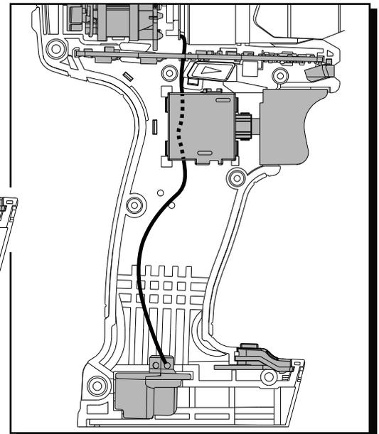
Solder the High Voltage Wire to negative terminal of battery connector block (along with black wire from switch). **Note:** Heat shrink tubing will have to be carefully trimmed away prior to soldering. After wire is soldered, wrap a thin piece of electrical tape around the two wires and terminal.
