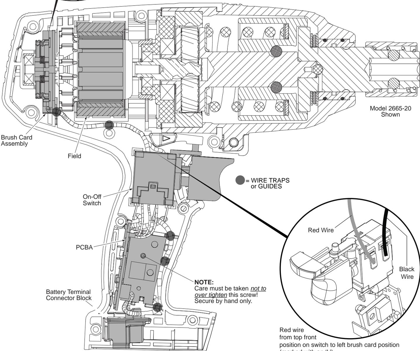
Red wire from top front position on switch to left brush card position (marked with an 'L').
