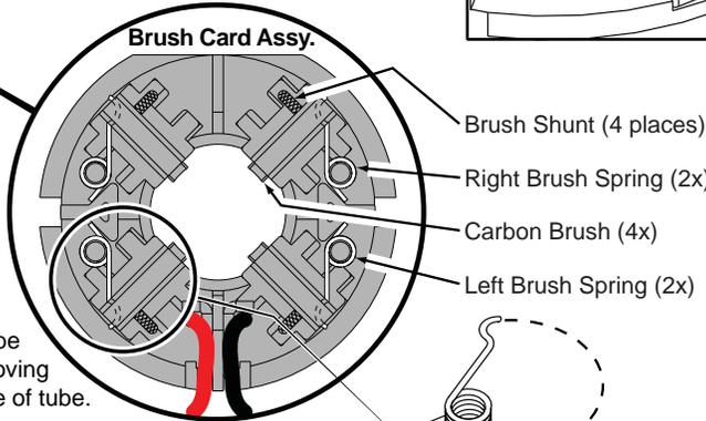
Be sure carbon brush is in brush tube with brush shunt moving freely in side groove of tube.
