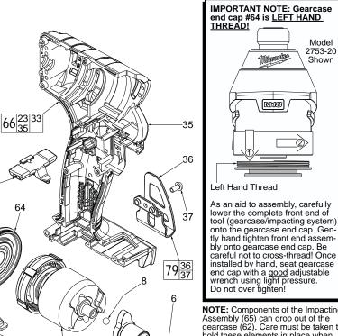
NOTE: Components of the Impacting Assembly (65) can drop out of the gearcase (62). Care must be taken to hold these elements in place when assembling onto gearcase end cap.
