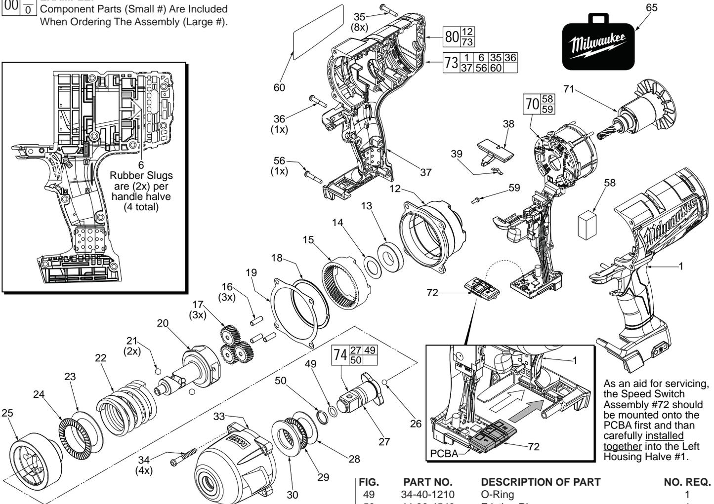
As an aid for servicing, the Speed Switch Assembly #72 should be mounted onto the PCBA first and then carefully installed together into the Left Housing Halve #1.
