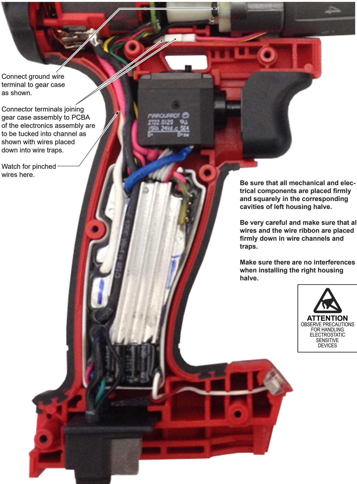
Connect ground wire terminal to gear case as shown.
