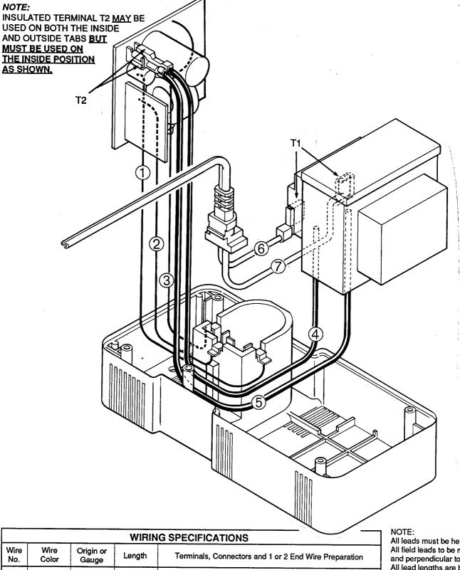
Wire No. 1 Red 22 Ga. Component of circuit board assembly. 4-1/2" 2 Red 22 Ga. 3-3/4" Component of circuit board assembly. 3 Red 22 Ga. 2-1/4" Component of circuit board assembly. 4 Yellow 20 Ga. Strip 1/4" for T2. 6" 5 Yellow 20 Ga. 6" Strip 1/4" for T2. 6 Black 18 Ga. 1-1/2" Strip 3/16" for T1. 7 Black 18 Ga. 3" Strip 3/16" for T1.
