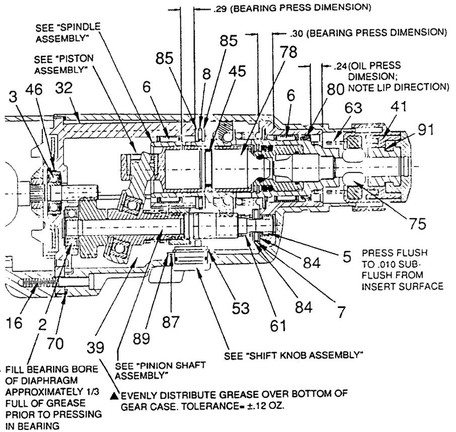
▲ FILL BEARING BORE OF DIAPHRAGM APPROXIMATELY 1/3 FULL OF GREASE PRIOR TO PRESSING IN BEARING
