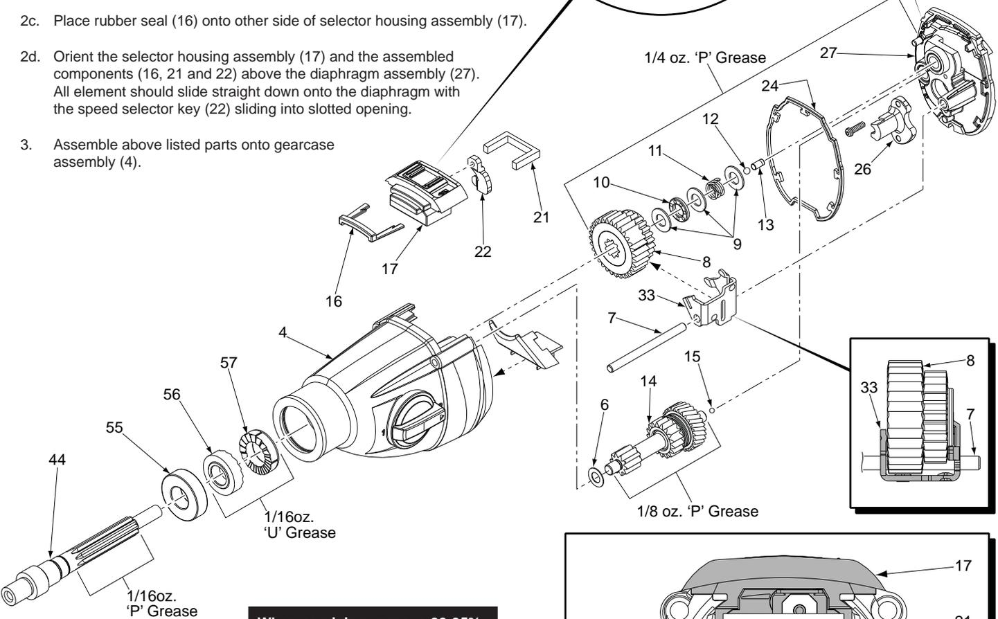
**When servicing, remove 90-95% of the existing grease prior to installing Type 'P' grease. Original grease maybe similar in color but not compatible with 'P'.**
