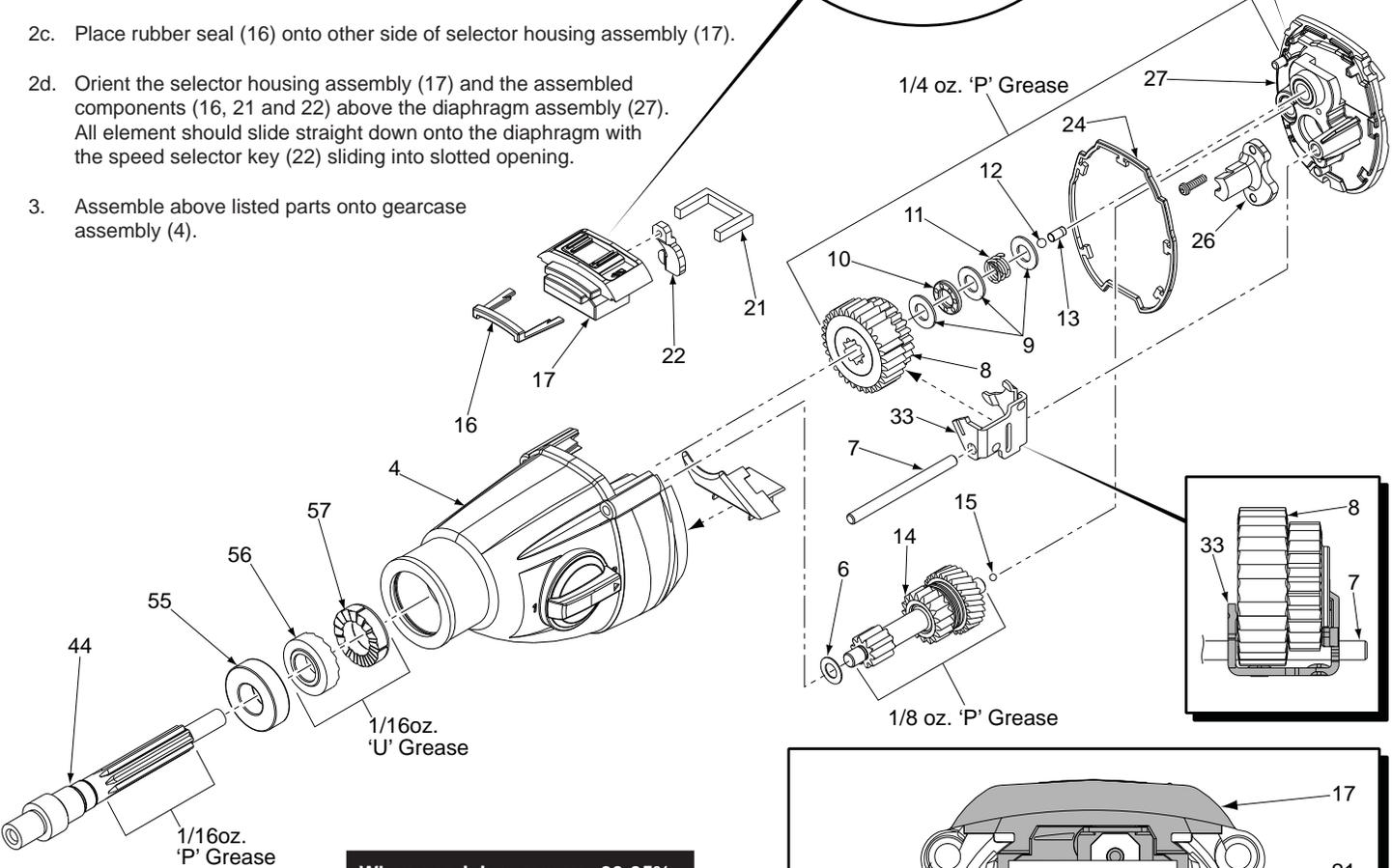
**When servicing, remove 90-95% of the existing grease prior to installing Type 'P' grease. Original grease maybe similar in color but not compatible with 'P'.**
