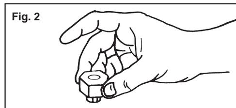
Position nut squarely over collet with the smaller opening of the nut facing up (Fig. 2).
