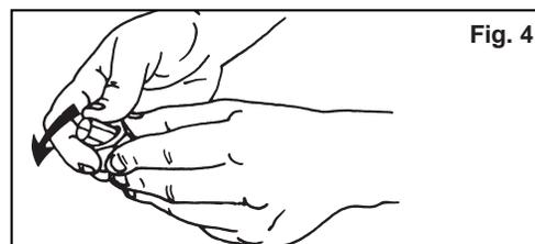
To remove collet from nut, hold nut firmly with one hand and press the collet to one side with the other hand (Fig. 4).
