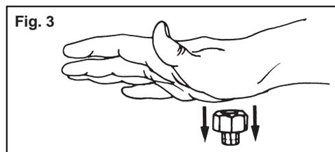
Snap nut and collet together by firmly applying downward pressure into assembly with palm of hand (Fig. 3).
