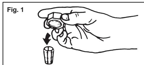
To assemble, place the narrow end of the collet on an even surface. Take the nut and place it over the collet (Fig. 1).
