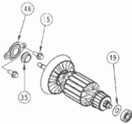
**31-50-1752 Motor Housing Kit** incorporates changes to the shielding of the armature pinion and commutator ball bearings along with the retaining of the pinion ball bearing into the gearcase assembly of 7"/ 9" 15Amp Sander / Grinders - 6080-20, 6081-20, 6082-20, 6086-20, 6088-20 and 6089-20.
