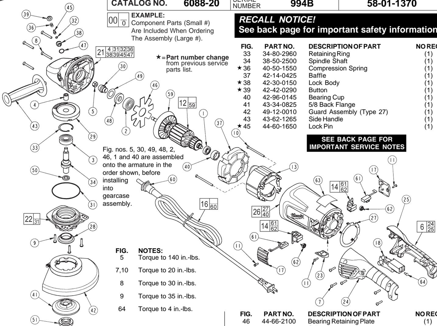
Fig. nos. 5, 30, 49, 48, 2, 46, 1 and 40 are assembled into the order shown, before installing into gearcase assembly.
