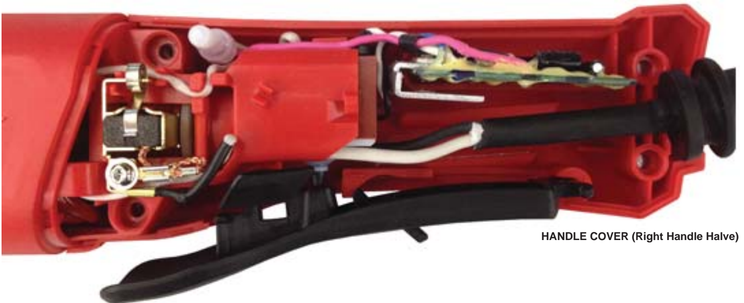
HANDLE SUPPORT (Left Handle Halve) Install all components and route wires here before securing with Handle Cover.
