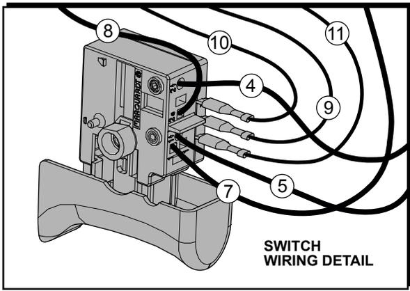
AS AN AID TO REASSEMBLY, TAKE NOTICE OF WIRE ROUTING AND POSITION IN WIRE GUIDES AND TRAPS WHILE DISMANTLING TOOL.
