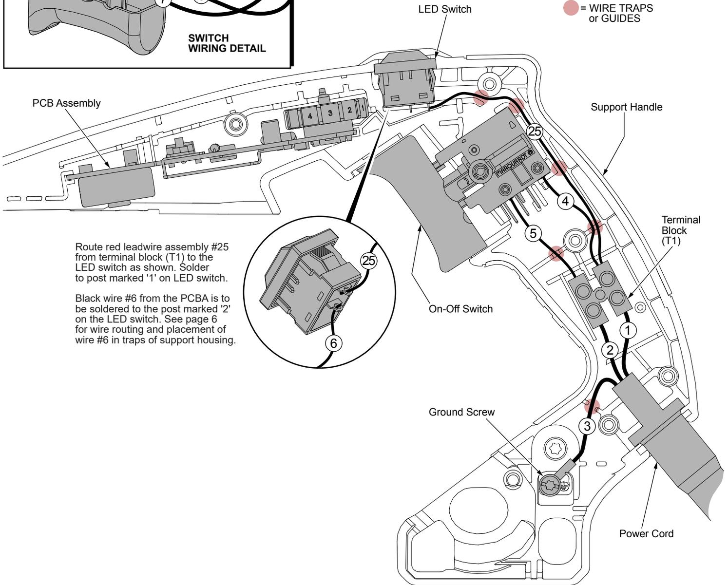
Route red leadwire assembly #25 from terminal block (T1) to the LED switch as shown. Solder to post marked '1' on LED switch.
