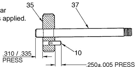
33,38 Press rear spindle bearing flush to .030 below bearing boss of diaphragm.
