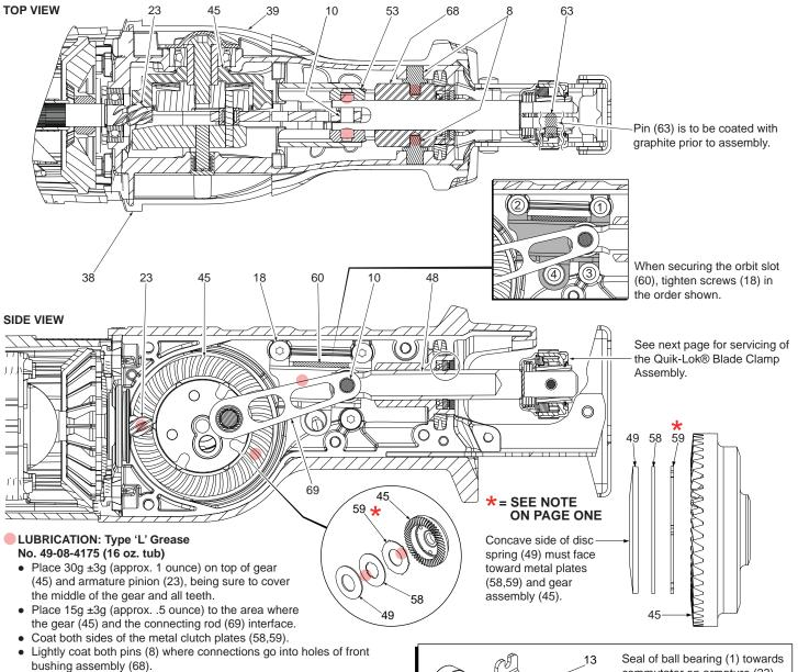
• Lightly coat both ends of pin (10) prior to installing rollers (53).
