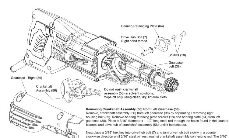
hex key can now be forcibly turned <u>counter clockwise</u> to loosen and remove drive hub bolt (7).
