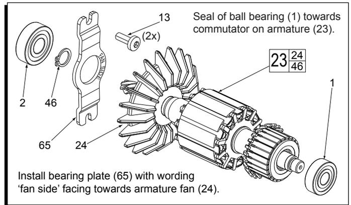
Seal of ball bearing (1) towards commutator on armature (23).
