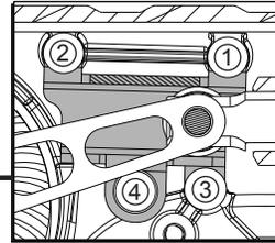
When securing the orbit slot (60), tighten screws (18) in the order shown.
