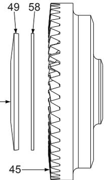
Concave side of disc spring (49) must face toward metal plate (58) and gear assembly (45).
