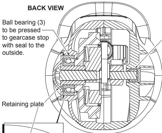
Ball bearing (3) to be pressed to gearcase stop with seal to the outside.
