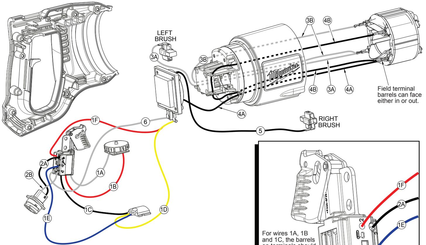
Field terminal barrels can face either in or out.
