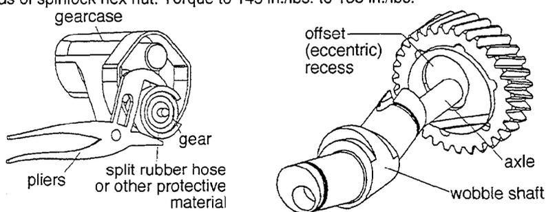
**REMOVING THE KEYLESS QUIK-LOK BLADE CLAMP**
