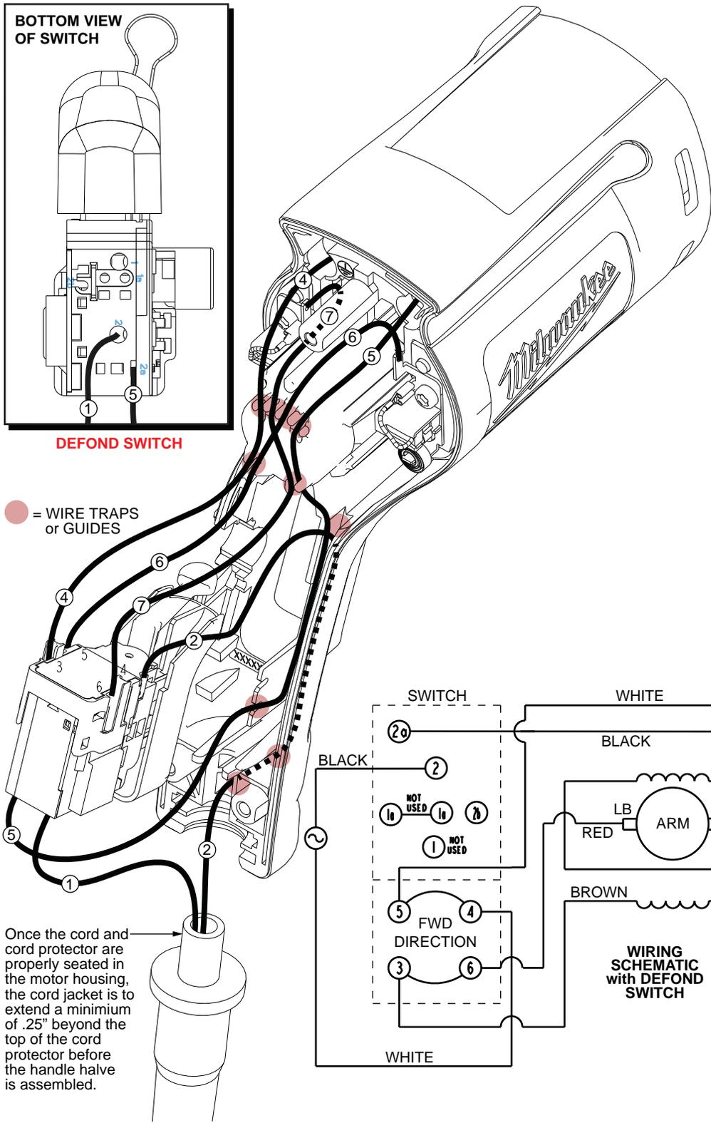
Once the cord and cord protector are properly seated in the motor housing, the cord jacket is to extend a minimum of .25" beyond the top of the cord protector before the handle halve is assembled.
